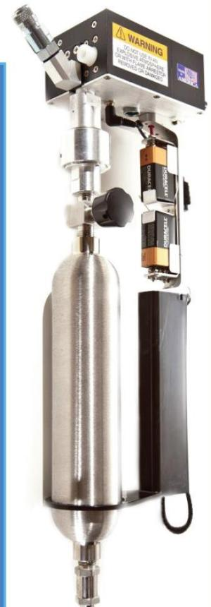
Flame Pack Shown without Probe Assembly and Battery Cover
