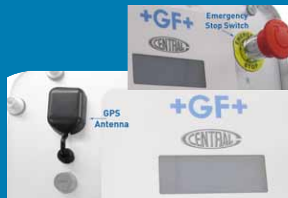
Emergency Stop Switch and GPS Antenna
