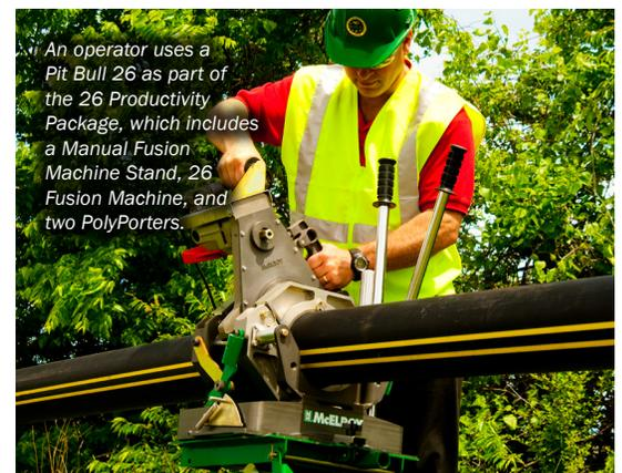
An operator uses a Pit Bull 26 as part of the 26 Productivity Package, which includes a Manual Fusion Machine Stand, 26 Fusion Machine, and two PolyPorters.
